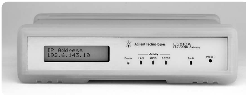
Figure 5. The Agilent E5810A LAN/GPIB Gateway and the 82357A USB/GPIB Converter.
